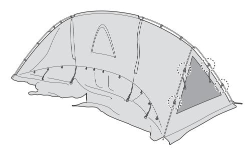
6 Gradually join the C pole ① with black ends at both tips and pass it through the sleeve with the black tape.
