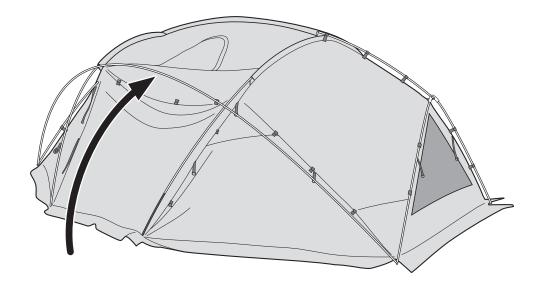
Secure the intersection of the C pole ① and C pole ② using the Velcro attached to the main body. When doing so, pass the Velcro through them so that the two poles are bundled together. (2 locations)
