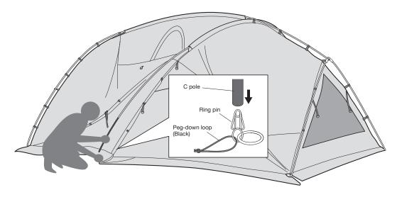
8 Extend the C pole ②, securely connect the joints, and insert the ring pin at the tip of the A pole into the C pole ②. (2 locations)
