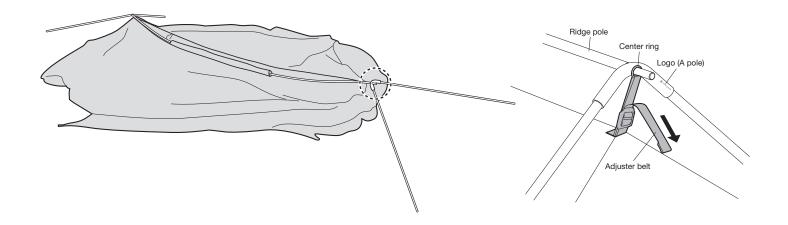
Insert the ring pin with the gray peg-down loop at the hem of the main body (triangular window) into the tip of the A pole. Attach it to the tip of the A pole and pull the adjuster belt to apply tension. Perform the same procedure on the other side.
