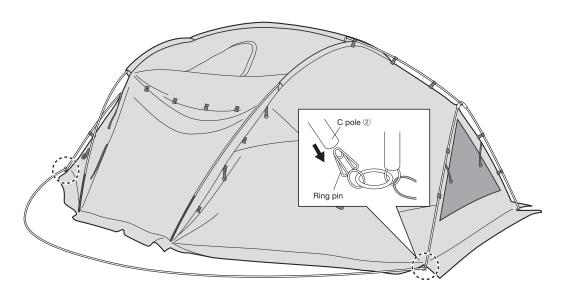
(9) Lift up the C pole ② and attach all the plastic hooks along the line connecting the C pole ② and C pole ①. (15 locations)
