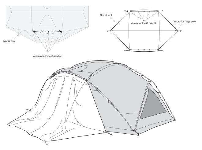
As shown in the figure below, cover the ceiling of the Merak Pro. main body with the shield roof, and wrap the Velcro for the C pole ② on the opposite side around the C pole ②.
