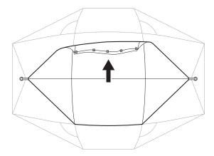
Wrap the Velcro for the ridge pole around the ridge pole to secure it.
