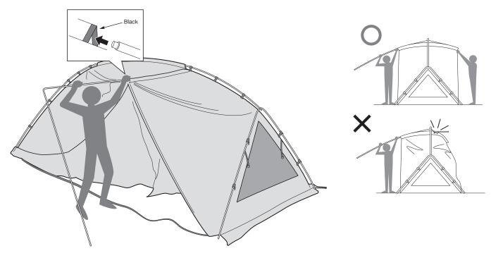
(7) Insert the ring pin with the black peg-down loop into the end of the C pole ①. Do the same for the C pole on the other side.
