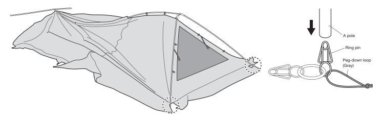
**5** Attach the plastic hooks along the line of the A pole to the A pole. (4 locations in each of the left and right sides) When doing so, check that the adjuster belt of the center ring ③ is not loose. If the belt is loose, adjust it to apply tension.
