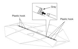
(3) Insert the tip of the ridge pole into the A pole joint. When doing so, ensure that the logo on the A pole is facing outward.
