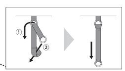
Wrap the belt with a ring around the C pole 2, attach the 5 m / 16.4' rope with a rope tensioner to the ring, and secure it using a peg.
