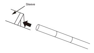
After passing the frame through the sleeve, insert the tip of the C frame into the ring pin on the outer side. Insert the other tip of the C frame the same way.
