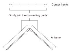
Check the part marked (see "Parts") and pass the center frame through the center sleeve.
