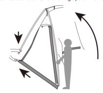
Extend the two C frames and then firmly join the connecting parts.
