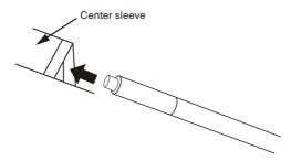
Connect the A frame to the ridge pole. Insert the ridge pole in such a way that makes the black sticker attached to the A frame face outward. Make sure that the tip of the ridge pole is inserted completely into the A frame.
