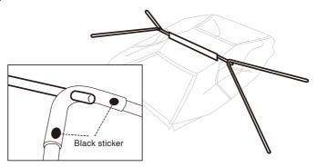
(5) Hook the center ring on the protruding ridge pole.
